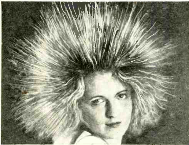
Fig. 1—A human electroscope. The similarly electrically charged hairs repel each other.
