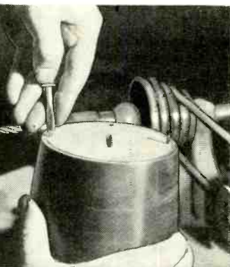
Six small screws hold the plywood false bottom in place.
