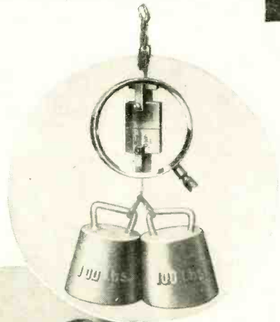
Above — Two Johansson gage blocks, accurate to four-millionths of an inch. Left—Model of Dr. Rumpler's proposed 180-passenger seaplane.
