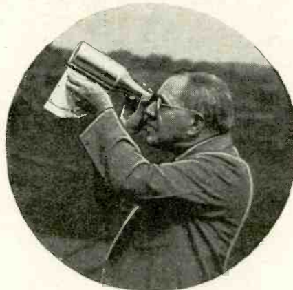
Above—Here's a queer-looking instrument, designed by Dr. C. F. Marvin, chief of the U. S. Weather Bureau. It is called a clinometer, and is used at airports to determine the height of clouds at night.
