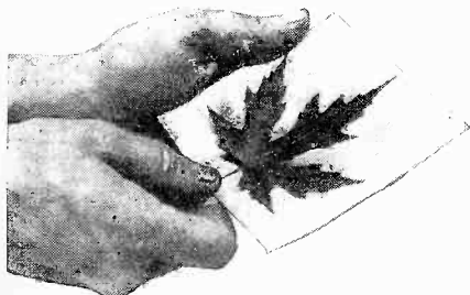
Hold a leaf against a sheet of paper prepared with luminous paint, then expose to the light; in the dark the outline of the leaf will appear as a luminous area.
