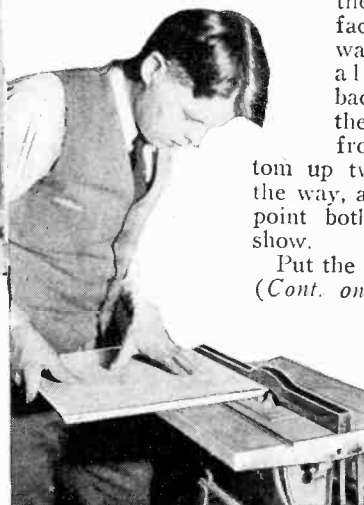
Cutting an edge on the molding cutter for the fourteen-inch-square top.
