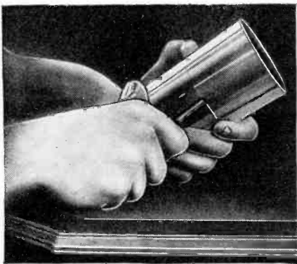
Scratching the scale mark on each glass simplifies tuning.
