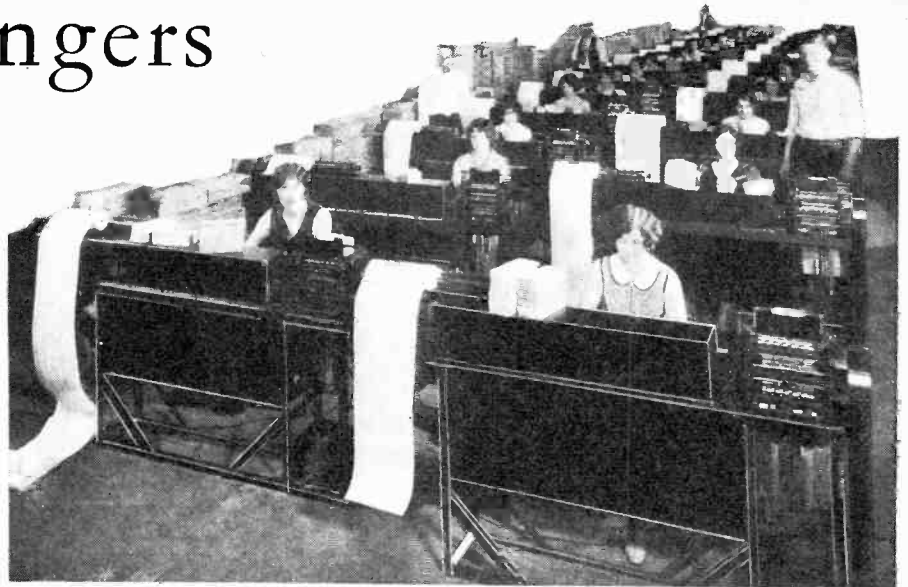
With electric machines these girls are totaling the information on the tabulating cards, 150 cards per minute.
