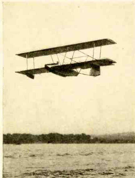
Glenn Curtiss made his hydro-glider flights in 1922 by the towed method.
