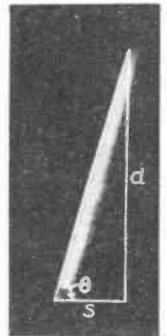
Figure 4—Method of calculating the speed of dynamite from photograph.
