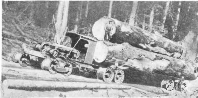
This 12-wheeled rubber-tired tractor hauls 60 tons of logs to the mills over pole rail tracks.
