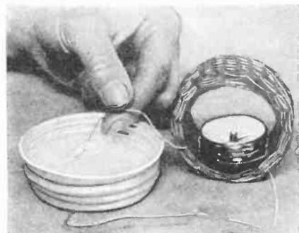
A zinc preserve jar lid containing vinegar, a honey-comb coil and a compass will make this miniature electric battery and galvanometer.
