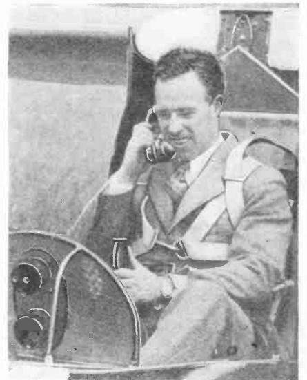
A line supported by a tow cable enabled Captain Hawks to hold the first conversation ever conducted over a wire between aircraft in flight on this cross-country trip. Here he is demonstrating how he phoned Jernigin.
