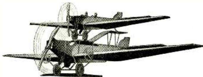
A plane fitted for a long flight often finds it difficult to get off the ground. In order to facilitate this, the smaller plane is mounted on a special platform built on top of a heavy lifting plane, is taken into the air, and released there.
