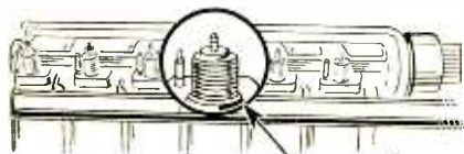
The valve gear of gasoline engines is a frequent source of trouble and stroboscopes are often used to investigate them. Sometimes, the valve will be seen to bounce two or three times before it comes to rest on its seat. This condition leads to broken springs.
