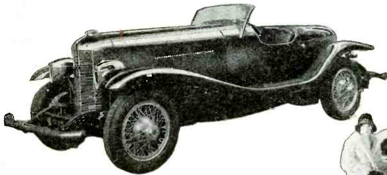
The photograph above shows one of the latest Dupont speed roadsters equipped with a 140 h.p. straight eight motor. At the left, is a two place Auburn cabin speedster, capable of maintaining a speed of 100 miles per hour, powered with a 125 h.p. straight eight motor. It is only 4 ft. 10 in. high and the body is made of aluminum material. The car with gas, oil and water included, weighs only 3,000 lbs.
