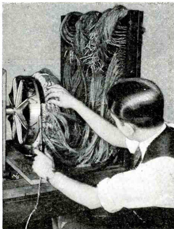
Fig. 3—The above photograph shows the complicated wiring of the transmitting board used by C. Francis Jenkins.
