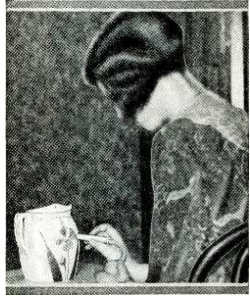
Fig. 6—This illustration shows how the air brush is used for decorating pottery and other small objects at home. Air pressure is supplied by pressing on the atomizer bulb.
