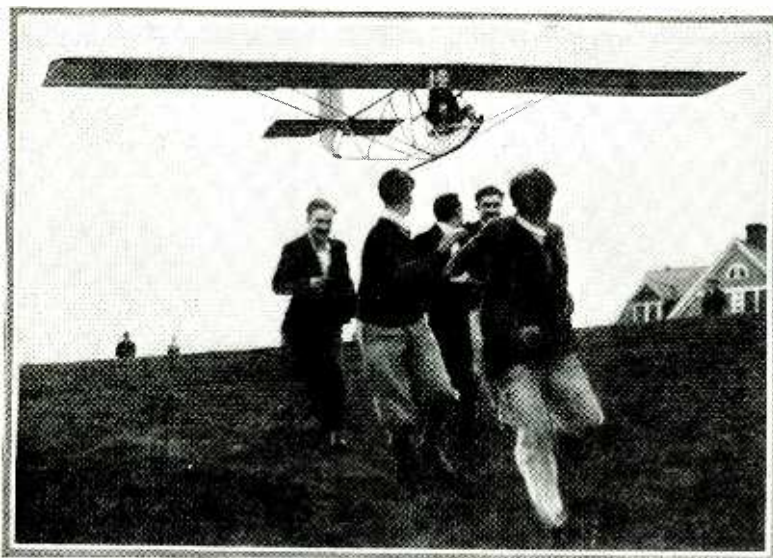
Fig. 3. The above photograph shows a glider similar to that described here but without the pylon. The group of assistants are launching the plane with a cable while they run downhill. This is one of the methods which can be used for getting the glider into the air.
