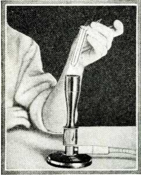
Fig. 1—Hold a one-inch tube in the flame of a Bunsen burner or of a gas stove, until the hole in one end has decreased in diameter until it is no larger than a small pencil.
