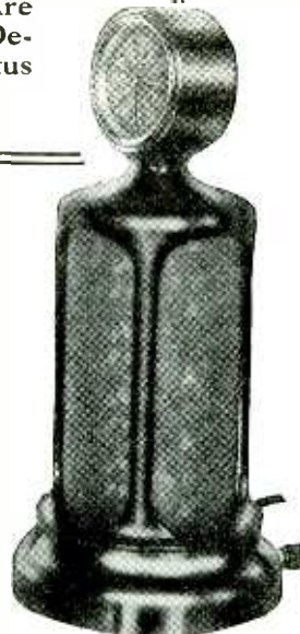
The clock shown above is a combined time piece, lamp and aerial.
