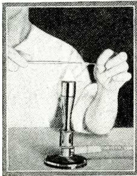
Fig. 2—This shows the second stage in the making of the air brush. A small tube is heated and drawn out and the opposite end is enlarged. The details of this can be seen in Fig. 3.
