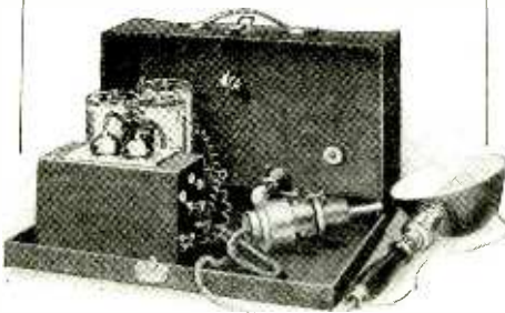
The above photograph shows one of the commercial stroboscopes which employ a neon tube and give remarkable results. The arrangement of an electric flash stroboscope is shown in Fig. 3.
