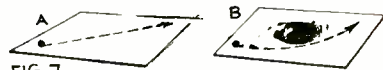
FIG. 7—The square at A represents a piece of tightly stretched rubber. If the rubber is flat a marble will roll "straight." If curved, the path of the marble will be curved but in each case, the path is a "natural one."
