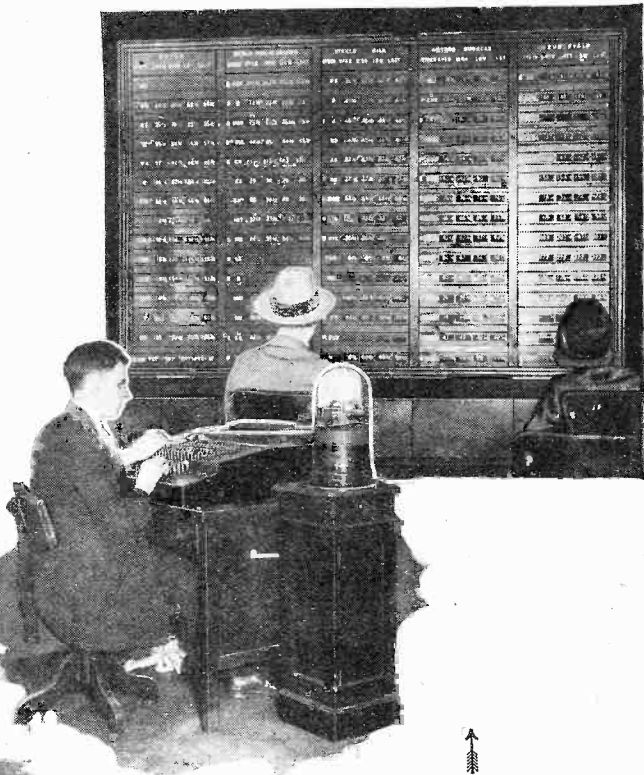
A newly invented stock quotation board eliminates the board box and is operated from a typewriter-like machine. The board shows the high, low and last prices of stocks just as given in the newspaper, and also tells if the market is strong or weak, by the flashing of a red or a white light.
