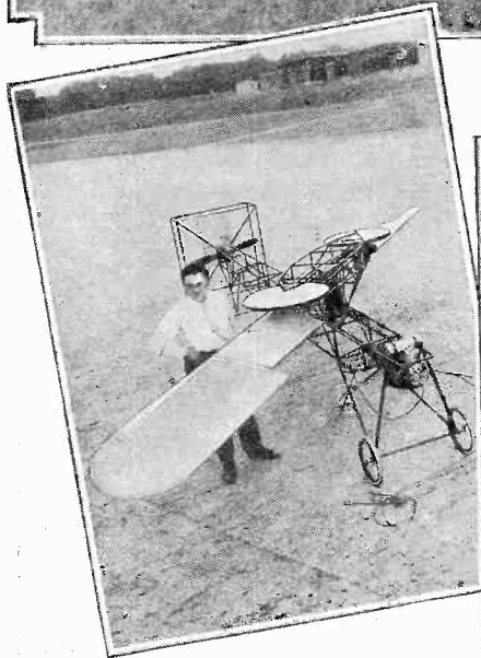
Prof. Zaschka, a German inventor, is shown above with a working model of his helicopter. This is expected to rise vertically from the ground and requires very little space for a take-off. This idea, of course, is not at all new and has been tried a number of times without much success. Helicopters were built which rose a short distance but were not capable of sustained flight. The inventor of this machine, however, is confident of success and is preparing to demonstrate at the Berlin flying field.
