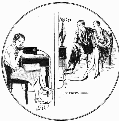
The drawing at the left shows how the tests are conducted, with the subject in one room and listeners in another. A foot switch is provided for cutting the microphone in or out of the circuit.
