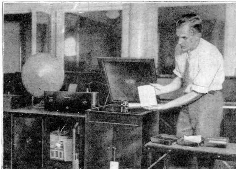
The apparatus above received Lindbergh's picture. The loud speaker was used for tuning the receiving apparatus to the wavelength of the airplane transmitter.
