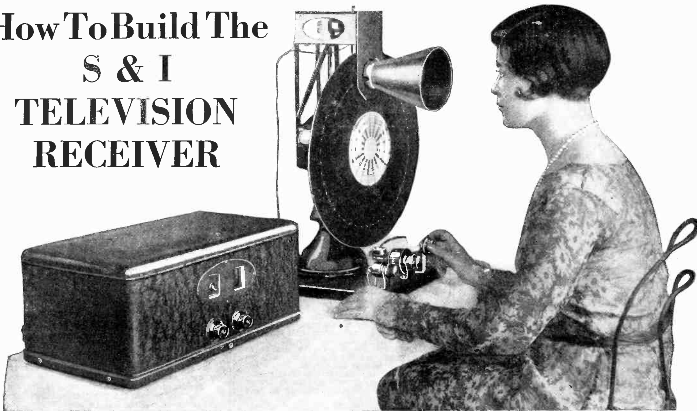
A slight adjustment of the rheostats and the picture comes in clearly. This photo shows a complete television receiver connected to an ordinary radio set. The picture is seen in the cone.
