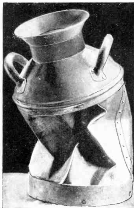
Above, we have a photo showing how the cream can was completely disrupted, owing to the vacuum created within.
