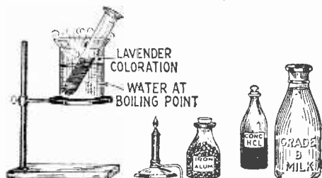
Fig. 1. A simple test to prove the presence of formaldehyde as an adulterant in milk.
