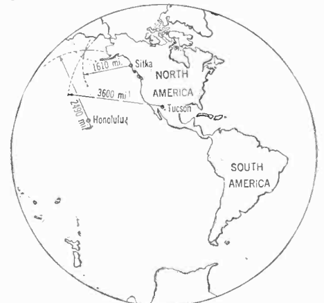
Above is a graphic chart showing method of locating earthquake by drawing arcs from three seismograph stations.
