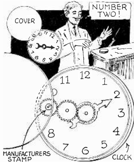
The arrangement of the gears for performing the X-ray eye effect is indicated above.
