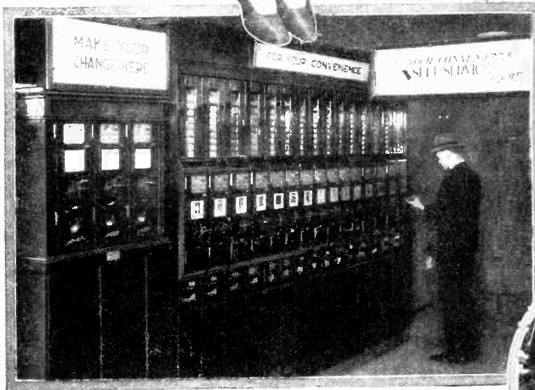
AUTOMATIC VENDING MACHINES —The above photograph shows the automatic merchandising devices recently placed into service in a United Cigar Store in New York City, where the customer can secure his package of cigarettes without waiting in line. Three machines make change, and then one drops the proper currency into the slot of the machine which distributes the cigarettes or cigars designated on the front of the panel.
