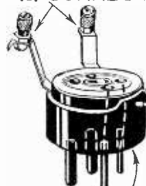
A new UX A.C. tube adapter is shown above. The A.C. connections are made to two lugs projecting from the sides.
