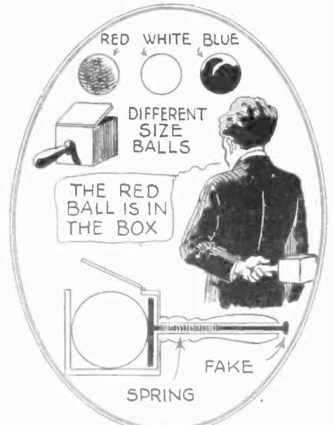
While the magician leaves the room, one of three colored balls is put into the ballot box which is closed. The other balls are concealed.
