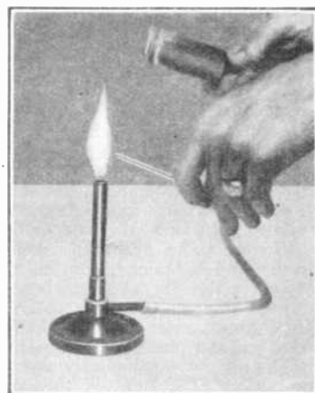
Chrome alum solution in bottle serves as a good flame color filter in flame tests for metals.
