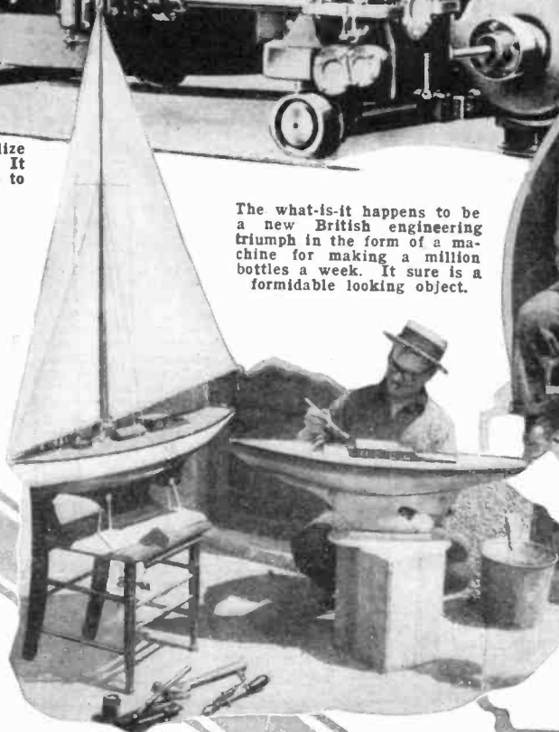
Axel Bisgaard builds boats of newspaper. The newspaper is cut up in the form of strips 1 inch wide and laid on a wooden form, after being wet. After this, layer is glued on layer until a shell containing about 30 thicknesses is formed. The entire shell is then removed from the wood, sandpapered, varnished, shellacked and fitted with deck and sails.
