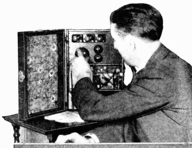
Above the receiver is shown in operation. It is practically a one dial control set as most of the tuning is done with the large variable condenser.
