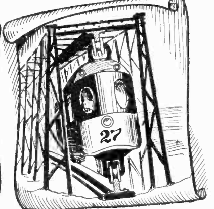
Railway used for many years near New York City. Had rails above and below.
