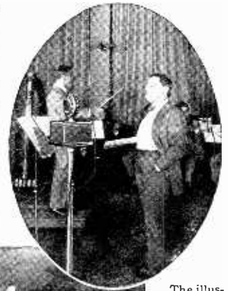
The illustration on the left shows the method used for recording for about 20 years. Note the instruments pointed towards the recorder.
