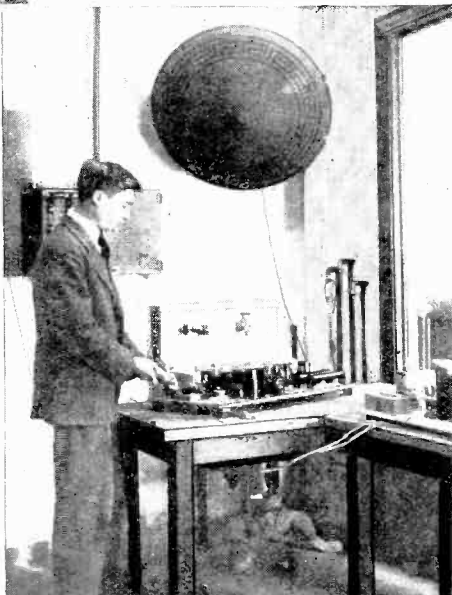
A charge is sent into the glass bulb containing the radium and the Alpha rays of the radium particle force apart the gold leaves of an electroscopical. The leaves are alternately discharged at regular intervals, thereby furnishing the energy operating the clock.
