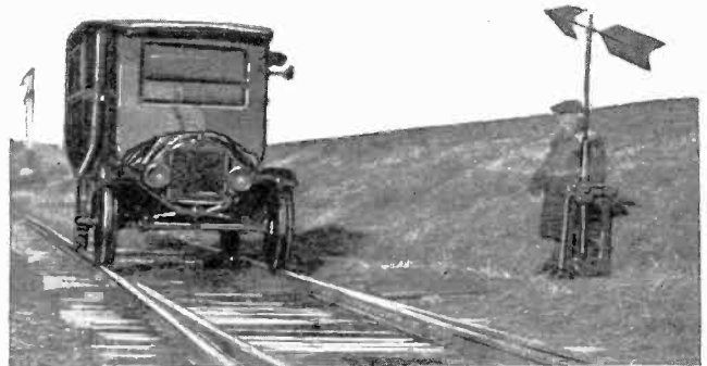
A new use for Ford cars. The car shown above has been equipped with a cab body and flanged wheels so that it may be run along the railroad tracks. The tracks provide a smooth roadway for the car which moves along under its own power.
