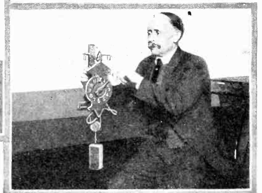
Carved by hand out of wood, this strange clock of ancient origin is still keeping excellent time for its owner. The "works" are composed of four wooden wheels and the pendulum is situated at the top of the time piece.
