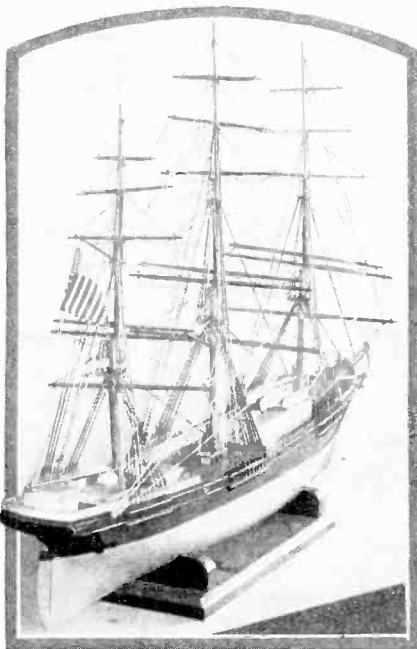
A view of the Benjamin F. Packard taken head on. This model is built to a scale of \frac{1}{8} th inch to the foot. Note hull lines.
