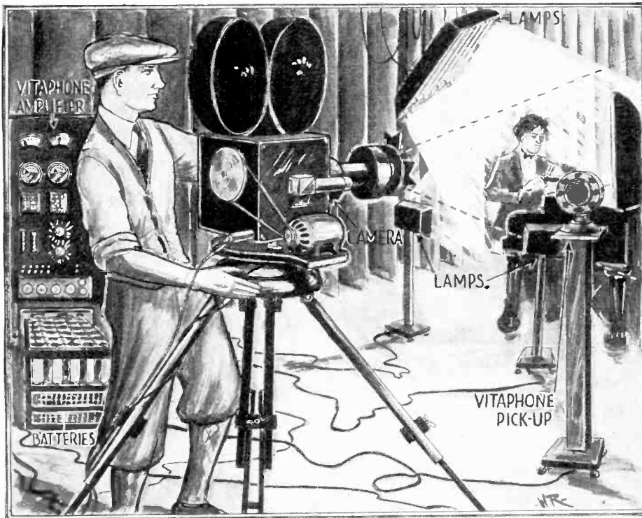
The method of photographing the actor or singer on moving picture film, as well as the recording of the voice, in the latest talking motion-picture known as the Movietone is illustrated in the picture above. The voice is recorded on the same film with the picture, as the other illustrations and accompanying text make clear.
