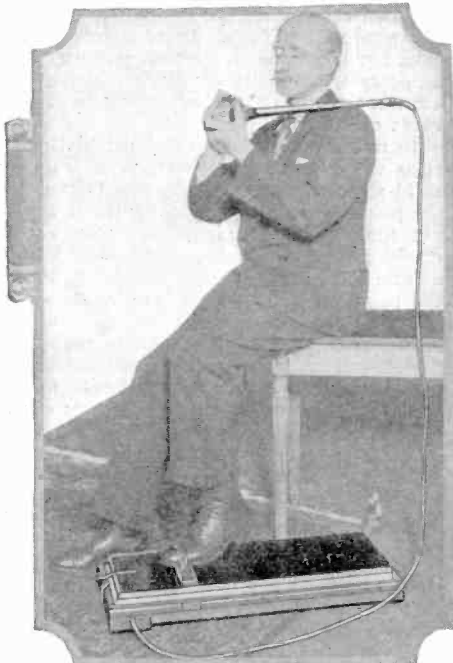
With a bellows, an organ pipe and his hands, Sir Richard Paget of England, shown above, has been able to say "Hello, London, are you there?" The bellows takes the place of the lungs, the reed of the organ pipe the vocal cords and the hands duplicate the mouth.
