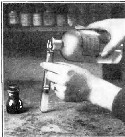
Aldehyde precipitates metallic silver. Above a silver nitrate solution is treated with ammonia until a clear solution is obtained.
