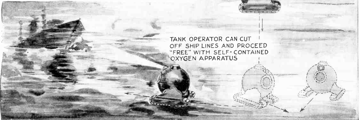
The above illustration shows the submarine tank in operation. It can either be connected to the mother ship at all times, receiving power and fuel supply or it may be cut free when desired. The illustration shows one tank being lowered into the water, and another at work.
