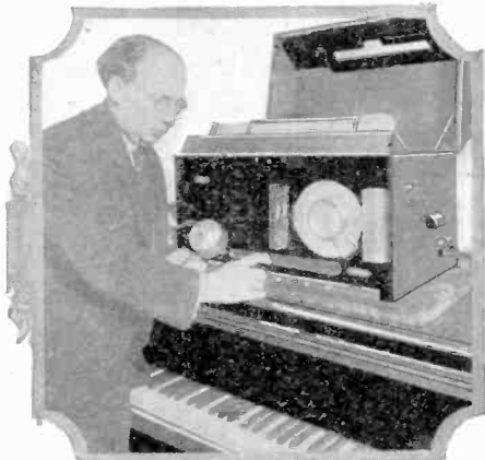
An instrument for measuring musical sounds and their synchronization has been invented by Carl Robert Blum of Berlin, Germany. The music film permits any rhythmic phenomenon, whether expressed in music, dance, or speech, to be recorded.
