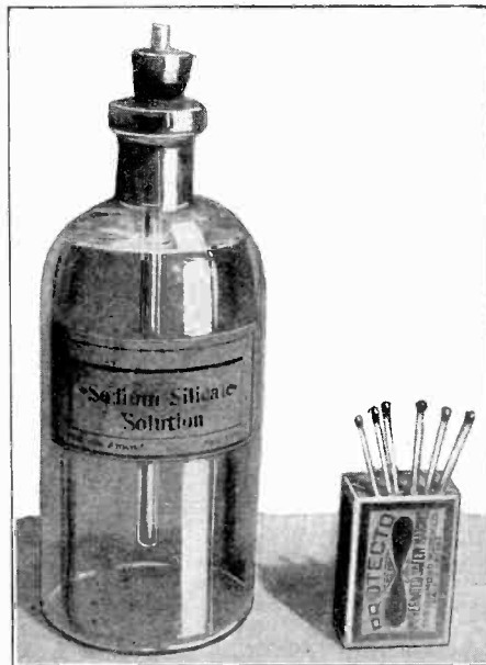
The ends of matches are dipped in sodium silicate solution and dried with disastrous results, as regards their future service.
