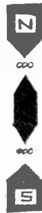
The illustration at the immediate left shows the relative positions of the magnet pole pieces and the moving coil. Note how the edges of the armature piece are tapered so that when the moving coil is lined up, a single line will join the points of the pole pieces and pass through the points of the armature piece.
