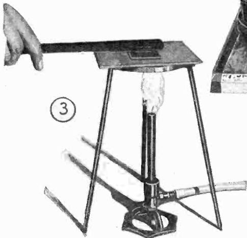
3. Smoothing off the melted selenium on the surface of the cell. 5. Testing the cell with a sensitive meter and a battery.
