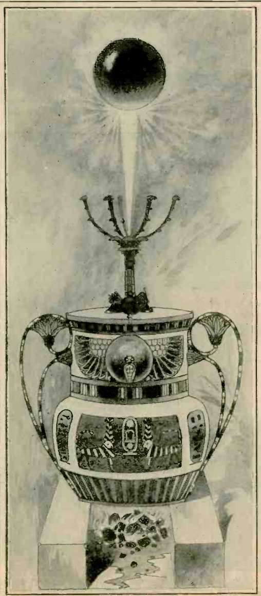
Directly below we see an illustration of the forty-fifth proposition of Hero's "Pneumatika" being a small boiler, maintaining a vertical jet of steam on the top of which a ball is supported and dances about. The device is most simple in operation, the large decorated urn is a container for water, and is heated by a fire, and steam, upon being generated, raised the ball from its basket-like cradle.
