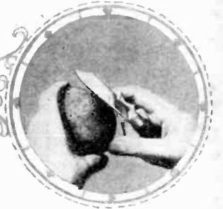
The sharp back of the average paring knife will often cut the hand of the user. The little metal device shown above protects this edge and prevents harm.
