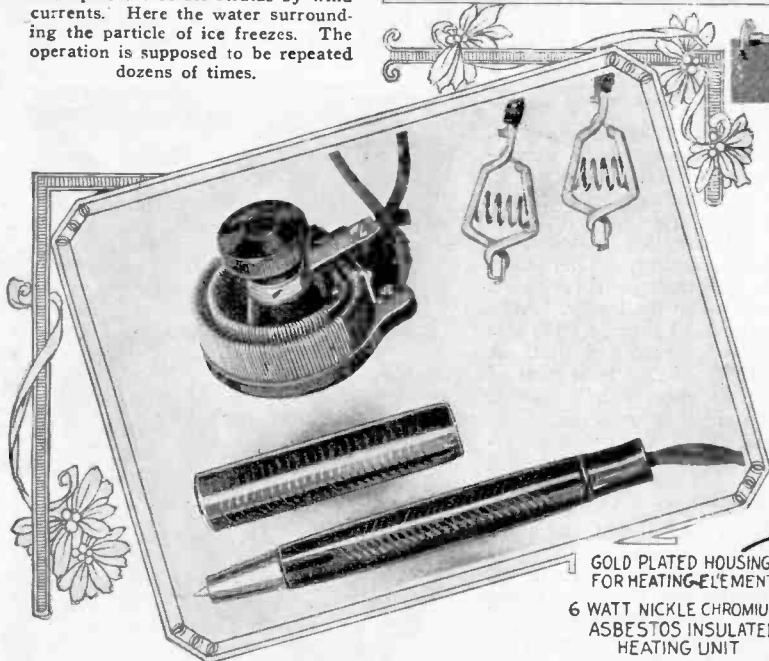
In the making of a fountain-pen for use in temperatures of fifty or sixty degrees below zero Fahrenheit, several interesting phases are presented. Heat is required surrounding the pen to keep it normally warm enough to accomplish the purpose, but not warm enough to over-heat the pen. The photo above shows the pen, the rheostat used to control the heat and the clips with which the leads are connected to the storage battery. Walls of metal with a thickness of .007 inch house the resistance wire between them. The pen tip projects just beyond the heater tube to prevent the ink from freezing there.
