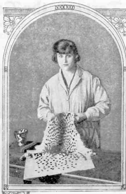
The photo at the left shows how artificial leopard skin is being made at the present time using the much maligned rabbit fur. A stencil is placed upon the rabbit skin and then an aniline dye is used to produce the spots. After the stencil is removed, the fur appears as indicated in the photo at the right. The fur can then be made into coats, or as was the style during the past year, it may be used to line or half-line a coat. Not only is the coat warm, but it is attractive as well. Milady ought to know, she was wearing a coat lined with imitation leopard fur last year.
