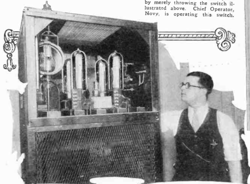
The heart of WRNY is shown at the left. Four large 250 watt vacuum tubes provide the power for putting this station over with a big "kick." Note the size of tubes as compared with the small receiving tube placed between them.
