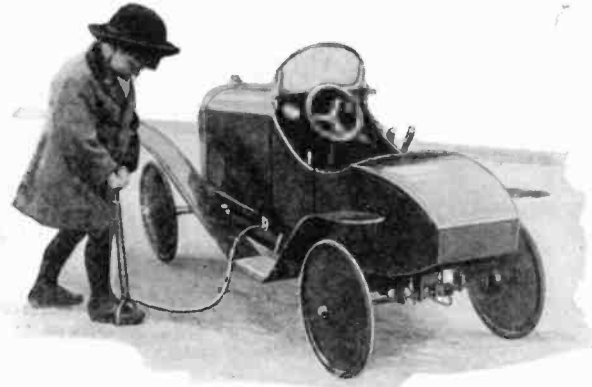
Above: Filling the compressed air tank by means of a hand pump. A pressure gauge on the dash board indicates the amount of power in reserve.
