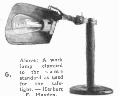
Above: Work lamp with half tin can as reflector.
