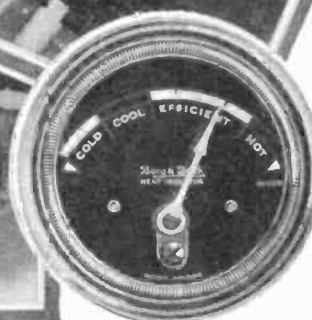
← On the automobile dashboard shown, there are two instruments; one indicating charge and discharge rates, gives the condition of the battery and when the button is pressed, it tells whether the battery is fully charged or weak. —J. W. Von Stein. The other tells whether the engine is cold or hot. The thermostat is clamped to the engine and the meter fastened to the dashboard. This is a better system than determining radiator temperature, because the latter does not give a true indication of motor heat. —Thomas W. Benson.
