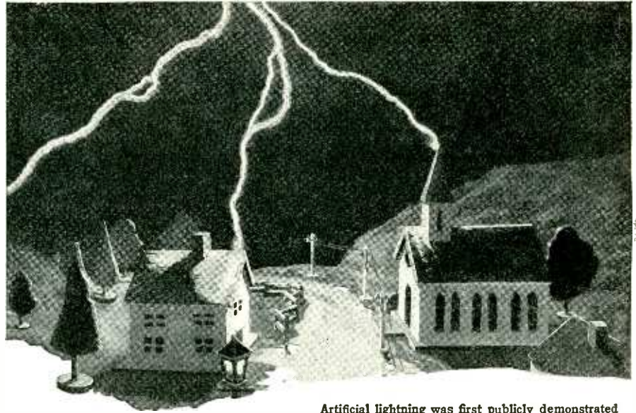
Artificial lightning was first publicly demonstrated on June 5, 1923, in the laboratory of the General Electric Company at Pittsfield, Mass., when a two-million-volt spark crashed into this miniature village.
