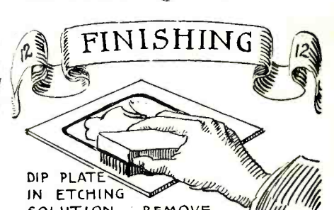
WASH ACID OFF AND REMOVE TINFOIL MOISTEN ASPHALTUM WITH TURPENTINE AND CAREFULLY SCRAPE OFF
