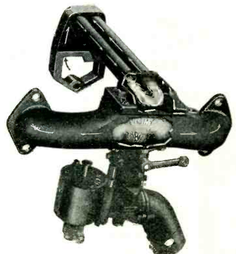
The automobile accessory illustrated above heats the vaporized gasoline before it enters the cylinders, causing more complete combustion.
