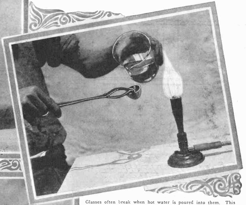
Glasses often break when hot water is poured into them. This is because the expansion of the glass with the heat of the water is so great that it is pulled apart. Some substances, such as pyrex, and quartz, expand very little when heated. For instance, a quartz vessel may be heated to redness and plunged into cold water without its breaking, because it expands very little with heat. The rate of expansion and contraction in a substance is known scientifically as its "coefficient of expansion."
