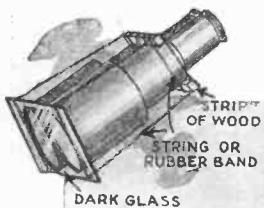
METHOD OF FIXING DARK GLASS ON FIELD GLASSES
