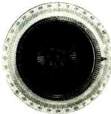
Tune for DX and CW Stations on the Same Condenser! A New Adjusting Knob, Known as the Univernier, Has Just Been Brought Out with Which It is Possible to Make a Closer Selection with a Regular .001 or .0005 Variable Than with the Use of a Vernier. By Means of Gears Inside the Knob Its Movement is Reduced Eight Times Making the Fine Tuning Possible. For CW Stations Slip the Knob in and It Works Directly to the Condenser Shaft Giving Broad Tuning and Quick Adjustment. Photo (Above) Shows Special Dial Graduated to Single Degrees for Use With the Fine Tuning.
