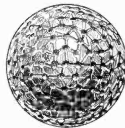
Mr. Vaile Suggests an Improved Design Above, Where the Indentations on the Golf Ball are Joined by Little Canals, so as to Permit a Fairly Continuous Passage of Compressed Air Around Either Side of the Ball.
