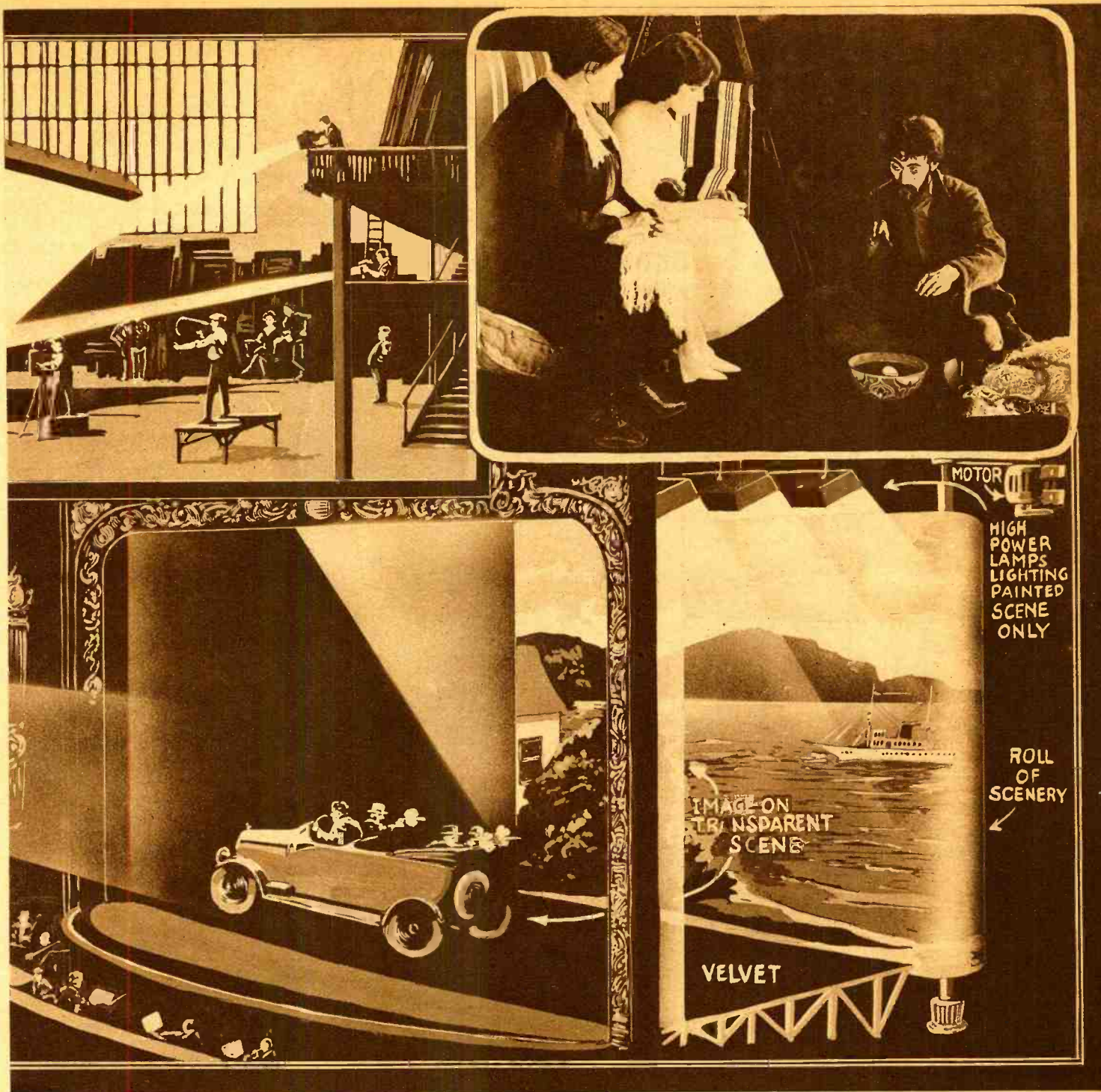
As Shown in the Illustration Above, the New French Perspective or Relief Movies are Projected on a Transparent Screen Placed in the Front of the Theatre Stage. The Background Scenery is Painted on a Canvas Strip, so as to be Rolled up, and the Successive Scenes are then Readily Moved into Position, by Turning the Rollers Either Manually, or by an Electric Motor Controlled from the Projecting Booth. The Insert Photo Shows How the Images of the Actors and the Furniture Appear in the Film, no Background or Floor Being Visible.
