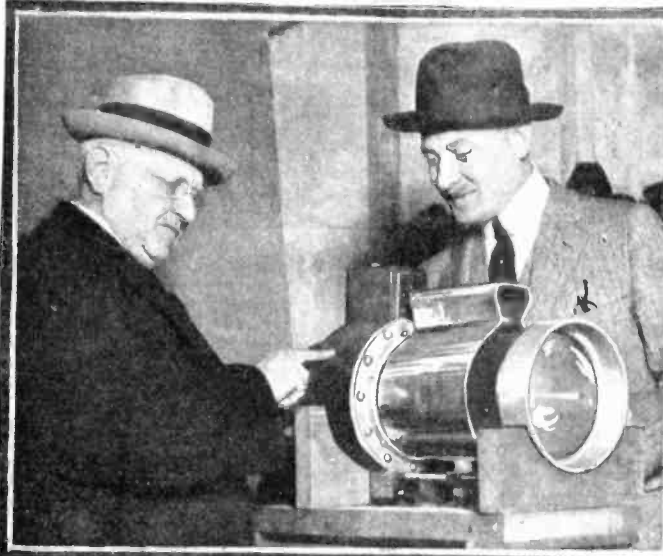
New "Cold Light" for Motion Picture and Stereopticon Projectors Uses But 6 Amperes Instead of 75 Amperes, as Do the Ordinary "Movie" Projectors. This Light Will Not Burn the Film No Matter How Long it is Left to Act and Will Save Cracked Lenses. The Inventor, M. J. Ritterath, is Seen at Right.
