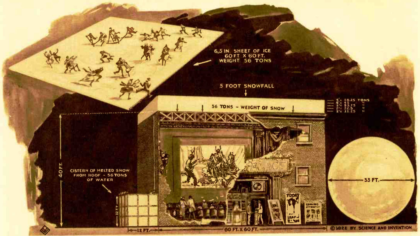
We Do Not Realize, Perhaps, What a Great Pressure a Roof Full of Snow Exerts on the Beams and Trusses, Frequently Causing the Roof to Fall In, as Did the Theatre Roof in Washington, D. C., Recently, When Nearly One Hundred People Lost Their Lives. Improper Design of the Walls and Roof Trusses, Careless Inspection or Poor Workmanship; Any One or All of These May be the Cause of Such a Roof Collapse, Except When a Phenomenal Fall or Drift of Snow May be the Cause
