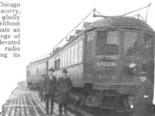
Top Photo Shows Antenna Wires Strung Along Roofs of "L" Train. Lower Left—Talking via Radiophone from Moving "L" Train in Chicago. Lower Right—Dancing to "Jazz" Music Received by Radiophone on Moving "L" Train.
