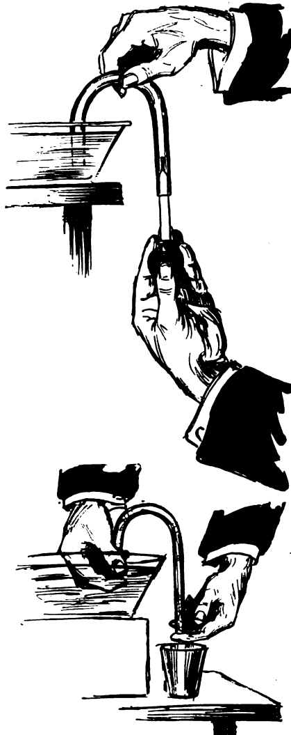
The Top Figure Shows How a Glass Pipette or Medicine Dropper May Be Inserted into a Siphon Tube, and a Partial Vacuum Formed by Squeezing the Bulb and Then Releasing It. The Lower Figure Shows How Oil or Other Liquid May Be Siphoned in a Dish or Pan With a Piece of Gas Pipe or Rubber Tube, Bent to the Shape Shown. This Tube is Filled With Liquid and Then Inverted, Removing the Fingers from the Tube Ends When the Shorter Leg is Under the Liquid in the Pan.
