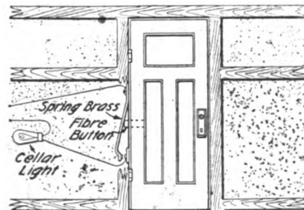
This Automatic Cellar- or Closet-Door Switch, Shown Greatly Exaggerated in Size, Will Save a Lot of Time and Cussing, for as Soon as the Door is Opened, the Light Flashes On.
