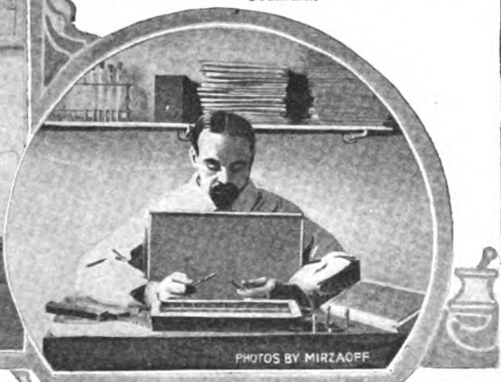
Apparatus Doubly Fitted With a Lead Screen, Showing the Operator Introducing Radio-Active Tubes Into Phials Which are to be Used for Experimental and Medical Purposes. Generally, Heavier Tubes are Used as Containers as These Filter Some of the Rays and at the Same Time the Tube Is Strengthened.
