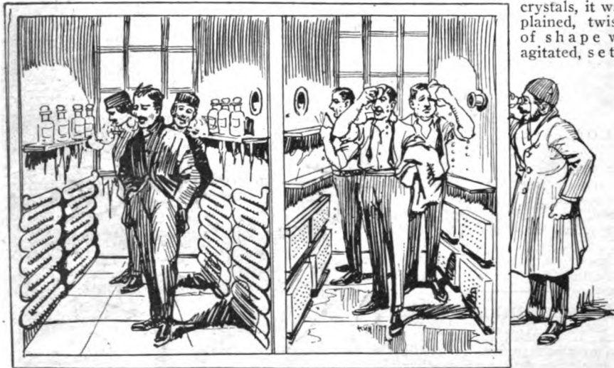
And Finally the Visitors Thought They Had Been Transported Suddenly to First the North Pole and Then to the Equator. Those Who Cared to, Were Allowed to Visit the "Hot" and "Cold" Rooms in Which Telephone Engineers Test Their Cables, Wires and Insulating Materials to Stand All Sorts of Rigorous Climatic Conditions. The Air Can Be Made as Damp as Desired in These "Bug" Rooms, as the Engineers Call Them.
