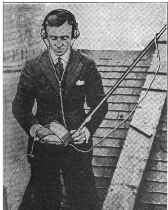
Captain Hyde A. Donisthorpe, of London, England, Has Recently Perfected a Very Ingenious Radio Receiving Set in Book Form, the Wave-Length Being Varied by Opening and Shutting the Book. Stations of Different Wave-Lengths Are Obtained by Opening the Book to Different Degrees, the Further the Book Is Opened the Longer the Wave-Lengths and Vice Versa.
