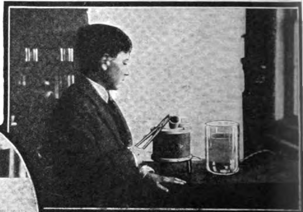
Removing the Crucible of Molten Brass from the Electric Furnace, Preparatory to Plunging It into a Jar of Cold Water.
