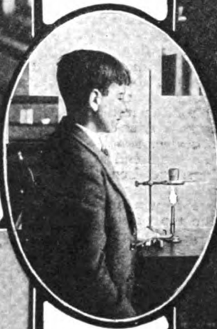
Below — Making Solder in the Chemical Laboratory. A Small Crucible Contains the Ingredients, Which Are Heated by Bunsen Gas Burner.
