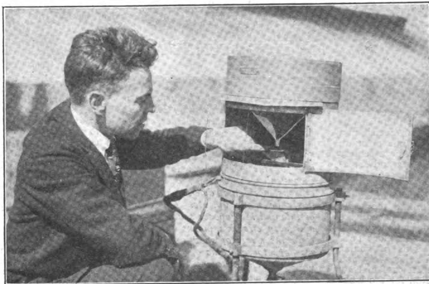
This Tipping Bucket Rain Gage—as the Delicately Balanced Bucket Shown at the End of the Operator's Finger Periodically Fills and Empties, Causes a Record to be Made on a Recording Drum. The Bucket Tips in One Direction or the Other, When Filled With a Quantity of Water Representing .01 Inch of Rainfall.
