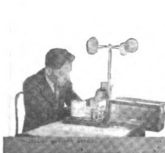
Two Important Factors in Forecasting the Weather Scientifically are "Air Pressure" and "Wind Velocity." The Barograph and Anemometer Read and Record These Quantities. The Four Cups of the Wind Speed Indicator and Recorder Rotate in the Breeze.
