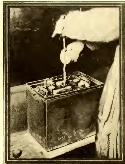
Filling the Battery According to Hoyle Does Not Need an Expensive Equipment. Water May Be Put Into the Battery Safely Without Spilling Over the Cells by Pouring Water From a Glass or Cup Down a Screw Driver Whose Tip Is Placed in the Cell to Be Filled.
