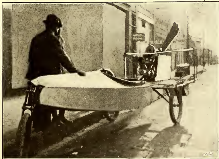
The "Hydro-Terra Firmamobile" is the Latest Device for Carrying Passengers Over Land and Water Out Vancouver Way. The Motorcycle Engine and Propeller Push the Outfit Over Land To the Tune of 70 Miles an Hour.
