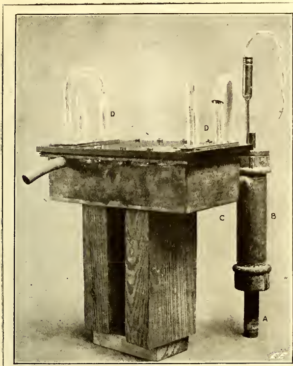
It Will Probably Come as a Surprise to Many That It Has Now Become Possible to Detect the Presence of Icebergs by Measuring the Amount of Salt in Currents of Sea Water. The Photo on the Left Shows the Apparatus Used for This Purpose. The Sea Water Is Pumped into "A," Passes a Resistance Thermometer in "B," into the Bath "C," and from There into the Electrolytic Cell "D," and Then Out of the Apparatus.
