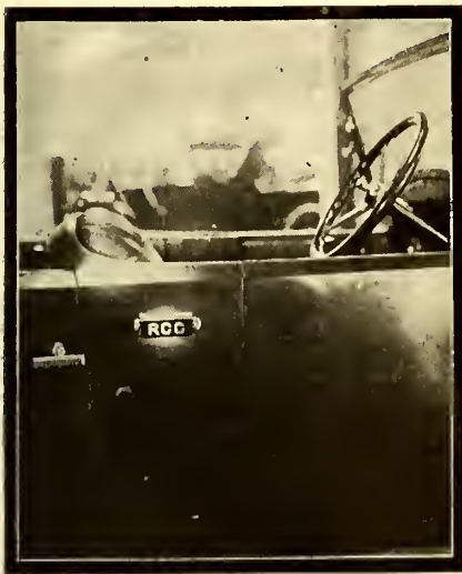
Here is the Newest Way of Identifying the Car—the Electrical Way. Electric Lights Shine Through Stenciled Initials in This Little Metal Device. Two Small Red Lenses Are at Either End of the Device Which Serve as a Standing Lamp for the Car. (On Use on New Fiat Car)
