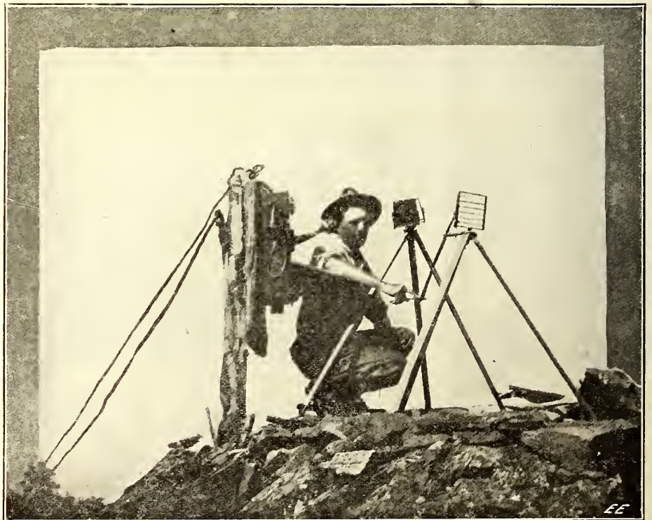
Science on the Mountain Tops—The Telephone and Heliograph or "Sun Mirror," Used in Signaling the News of Forest Fires in Our Great Timber Sections of the West and Northwest.
