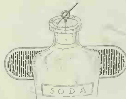
A Cork Screw in a Jiffy—Simply a Nail and a Screw Eye Do the Trick.
