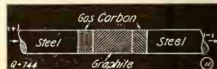
Compound Joint of Steel-Carbon-Grafito, Which, the Querist Desires to Heat Up Electrically.
