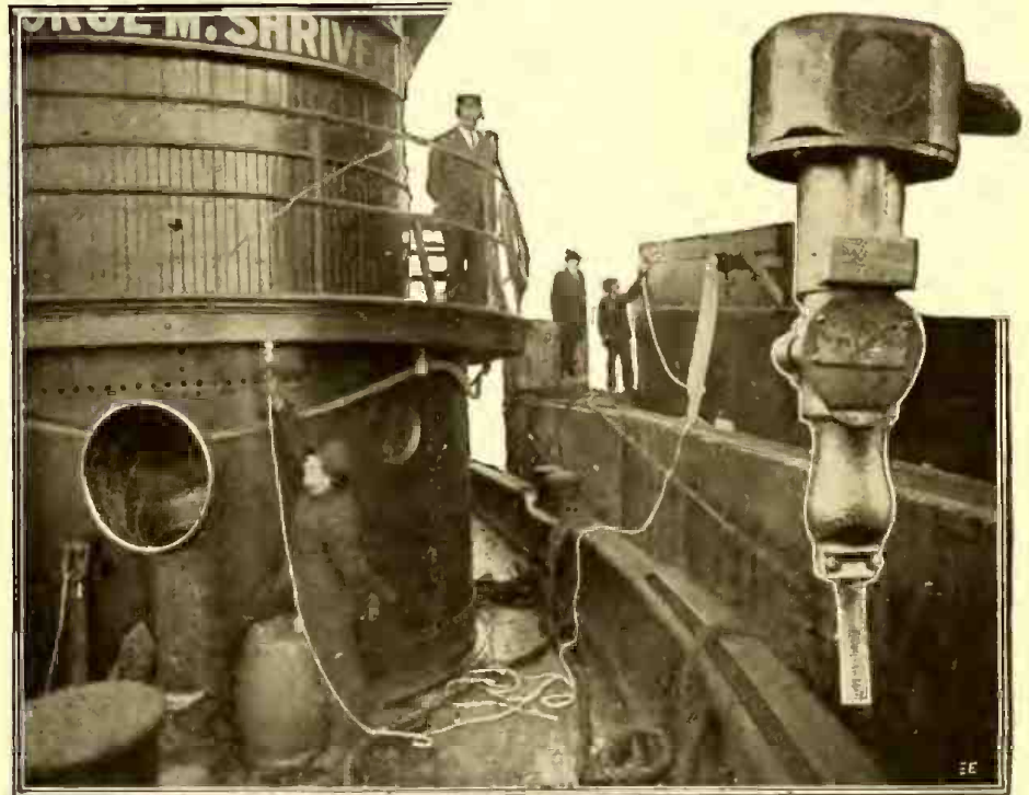
The Telephone Is Proving More Indispensible Every Day—Here We See It Adapted to the Requirements of Tug Dispatching At One of the Large Eastern Railroad Terminals. Connecting Jack On Pier Shown Enlarged At Right.
