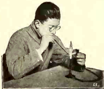
Fig. 61. How the Blow-pipe is Used in Chemical Work. A Bunsen Burner Supplies the Flame, a Part of Which is Blown out Sidewise by the Blow-pipe.
