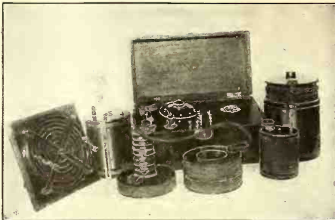
Photo Showing Several Types of Radio Inductances and Wave Meter as Used for Measuring the Value of the Inductance of Such Coils.
