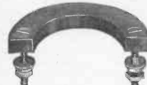
B Battery Potentiometer Unit
