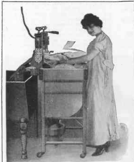
A Novel Electric Clothes Washer With a Capacity of 9 Sheets. The Revolving Cylinder is Shown in Upper Position for Convenience in Removing Clothes. A Motor-Driven Propeller Forces a Jet of Soapy Water Up Thru the Revolvable Cage Containing the Soiled Clothes.
