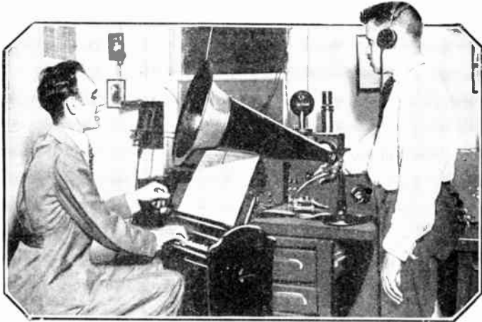
What an amateur music broadcasting station looks like. The horn conveys the sounds to the sensitive transmitter and vacuum tube
