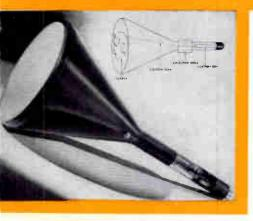
The Kinescope, corresponding to the "loud speaker" of an ordinary radio receiver. Diagram illustrates functioning.
