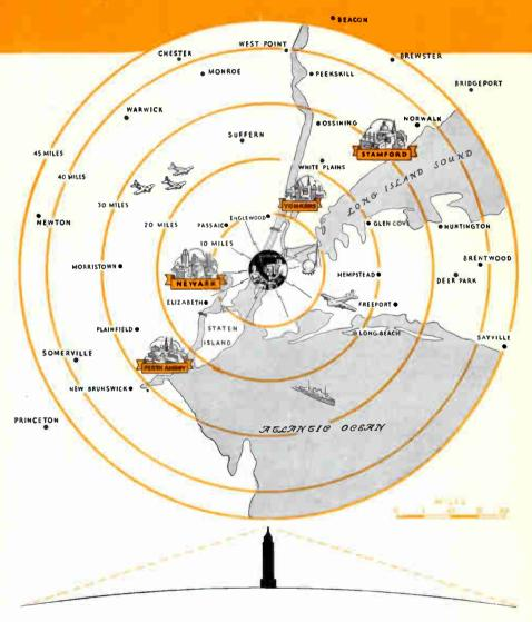
This sketch illustrates roughly how the altitude of a transmitting antenna determines the area served by a television broadcast. The point where the dotted line touches the earth is the horizon, the theoretical limit of dependable coverage. Roughly, the range of the antenna, 1300 feet above Fifth Avenue, is about as far as your eyes can see from that elevation. (The vertical scale of this sketch is greatly exaggerated.)
