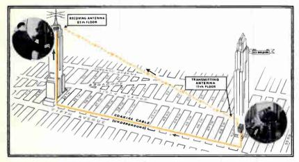
Sketch indicating how NBC television signals travel from RCA Building Studio 311 (right) to the Empire State Building transmitter (left). The solid yellow line represents a coaxial cable. Television picture signals may also be sent from studio to transmitter by radio waves, indicated by the broken yellow line.
