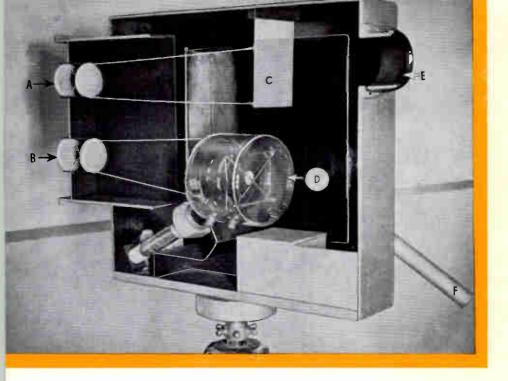
Simplified cutaway model of television studio camera, indicating principal parts.
