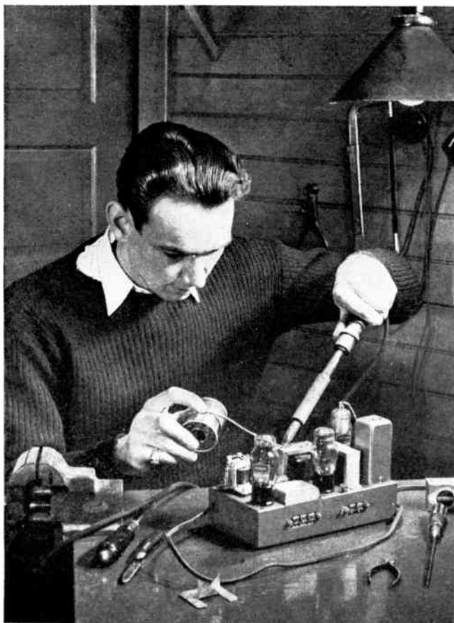
All connections must be soldered carefully, and a metal shield, as at the right, must be used to eliminate radio interference
