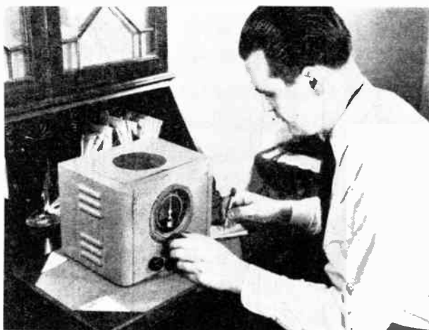
This two-tube superhet gives loudspeaker reception of local stations with a 20-foot antenna laid on the floor
