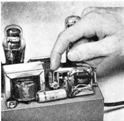
A close-up of the motor that turns the dual condenser
