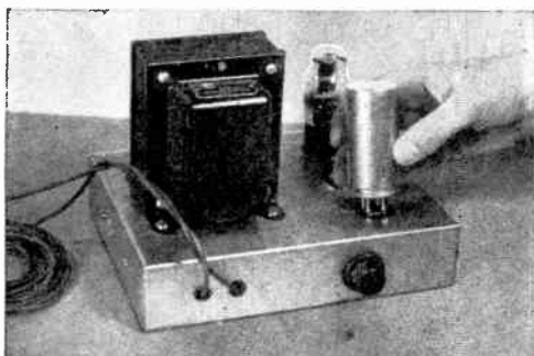
The vibrator is mounted on top of the chassis with the transformer, rectifier tube, and 110-volt socket
