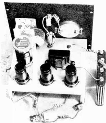
Tubes shown here are the new all-metal, 6.3-volt 6SJ7 type, but battery 1SA6GT tubes will serve
