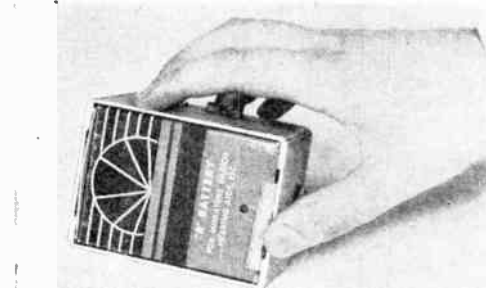
The 67 1/2-volt "B" battery that supplies plate current to all the tubes in the two units fits snugly in the bottom of the grey wrinkle amplifier cabinet
