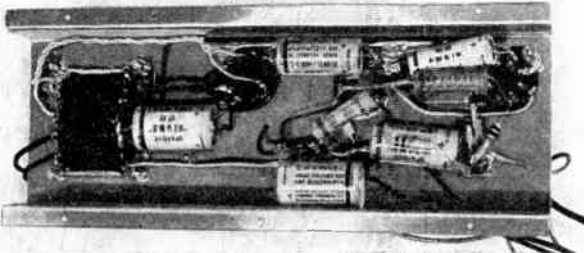
Top and bottom views of the amplifier chassis which should be bolted to the bottom of the suitcase under the motor-panel grill. Metal tubes are used—an important advantage in portable units
