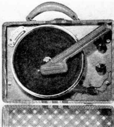
Completed phonograph seen from above, with eight-inch turntable. The seven-foot antenna is coiled
