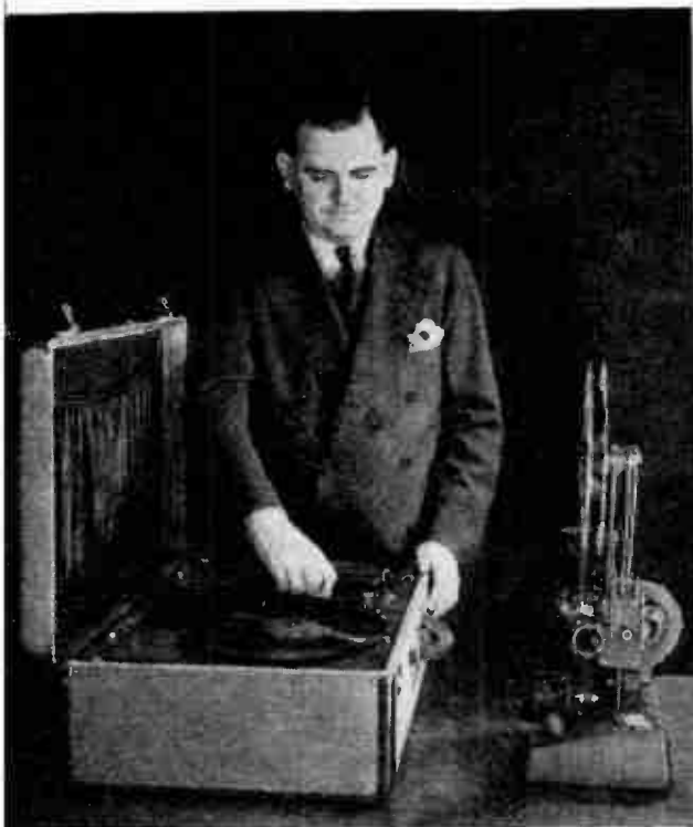
How the two units are set up for use. The phonographs are beside the movie projector where the operator can put on and change records and regulate the volume. The speaker unit, connected by a 25' cable, is placed near the screen
