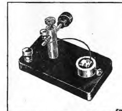
The Galena Crystal Requires a Fine Contact Wire.
