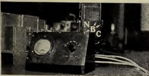
The applause and laughter of a typical studio audience such as the one portrayed on the right are measured by the "applause meter" shown above.
