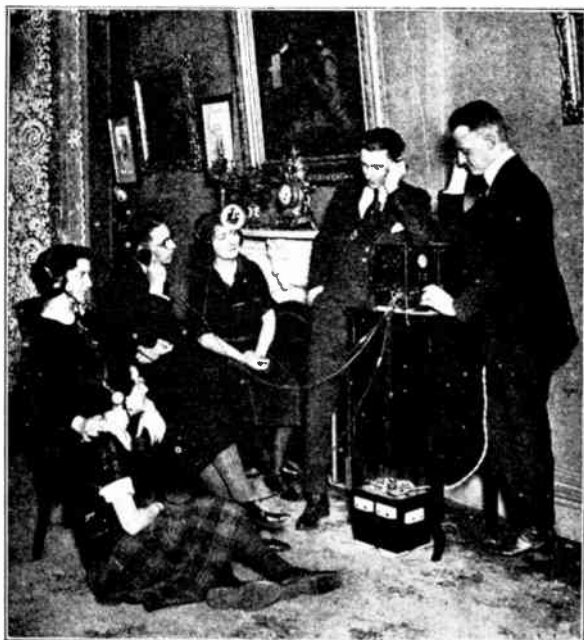
By using the four-point jack and double plugs illustrated here, many persons may listen in.
