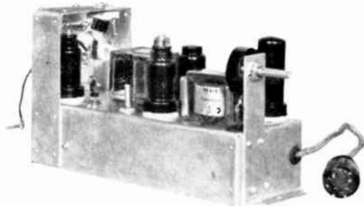
Fig. 129. Ultra-high-frequency receiver for police motorcycles
