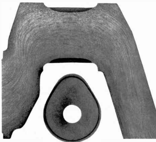
Fig. 97. Section of crankshaft with hardened bearing surface and a cam section hardened by inductive heating
