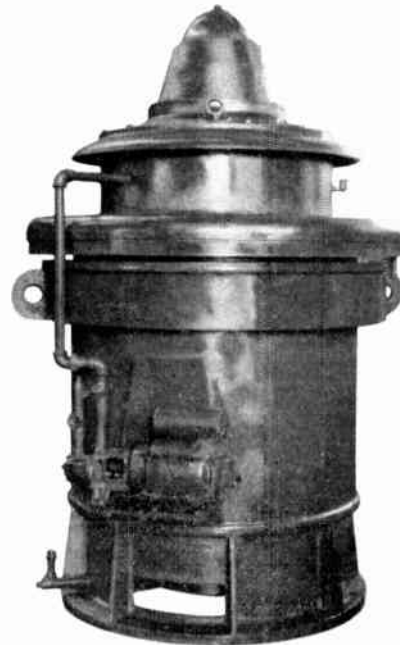
Fig. 74. A large vertical motor for mine dewatering
