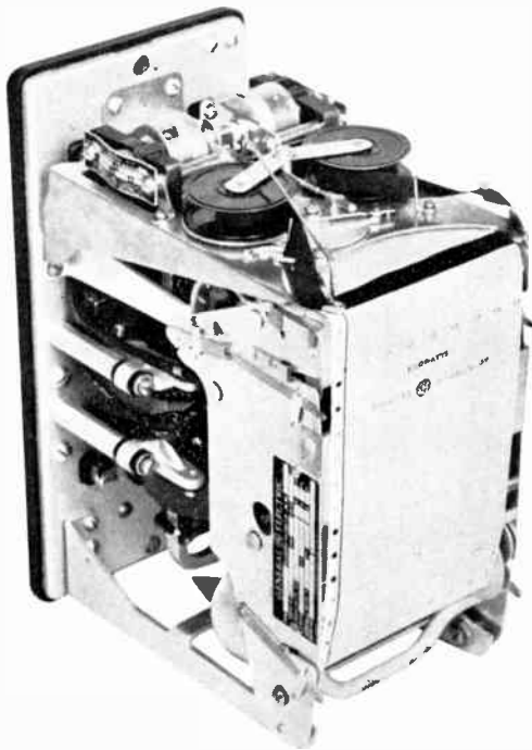
Fig. 42. Inkless-type recording instrument
