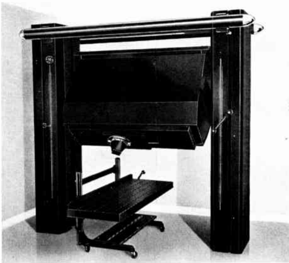
Fig. 134. Oil-immersed, self-contained 400-kv x-ray therapy equipment
