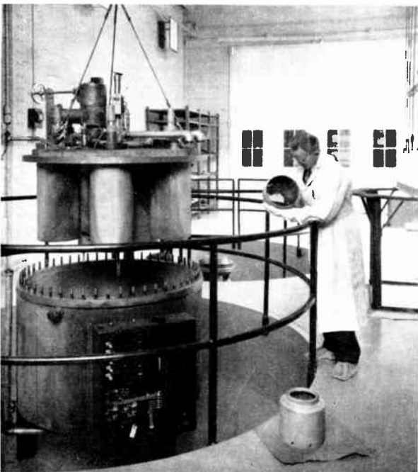
Fig. 52. Six-anode 1,000-kw metallic-tank mercury-arc rectifier being assembled. The centralized terminal board is shown on the side of the tank.
