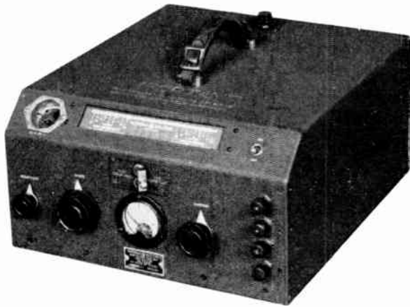
Fig. 45. Portable bar-to-bar test set
