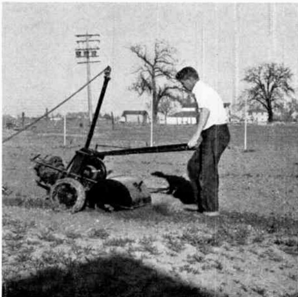
Fig. 140. A motor-operated cultivator for truck gardening and nursery work
