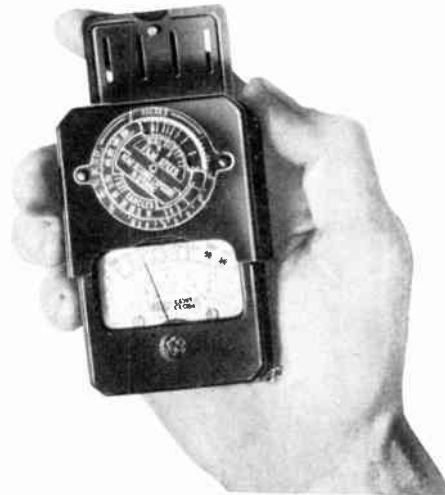
Fig. 47. Exposure meter for photographers
