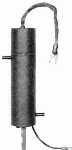
Fig. 55. Metal mercury-pool tube for welding control
