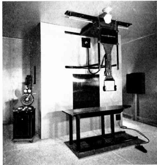
Fig. 136. Biplanar fluoroscope for localization and removal of foreign bodies from food and air passages
