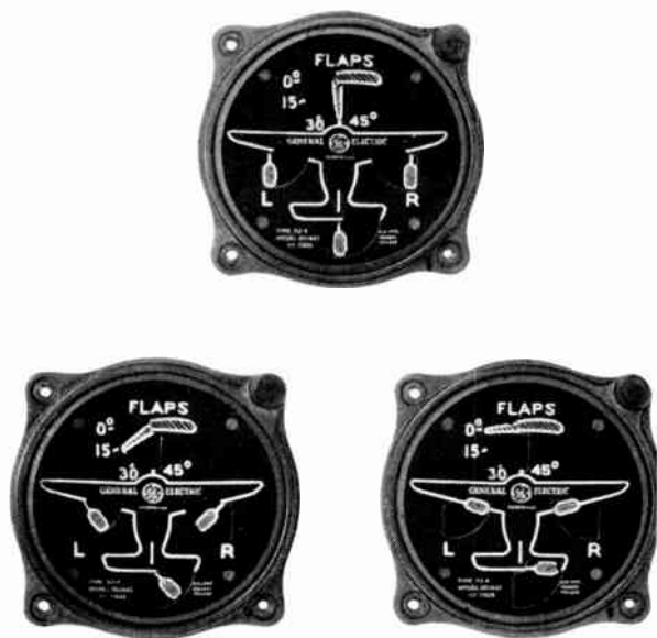
Fig. 71. Aircraft d-c Selsyn landing gear and flap-position indicator
