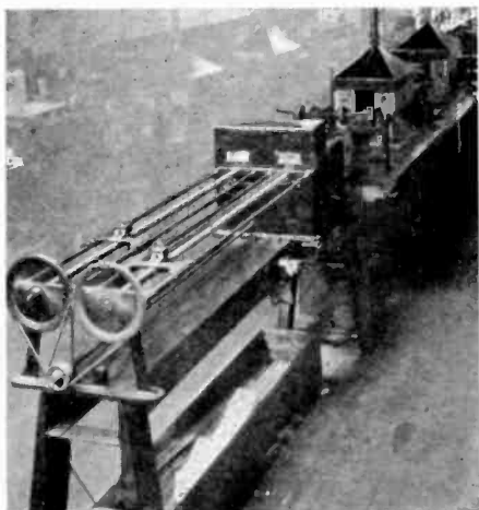
Glass-rod feed at front, next the drawing dies, the coating pads and last the baking oven.
