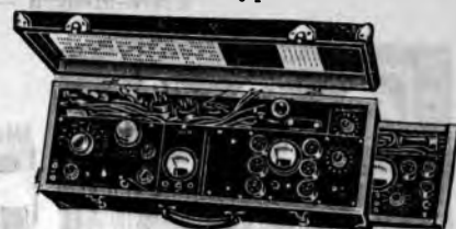
No. 576 Tube Tester, Tube-Short Tester (Set Analyzer Oscillator)
