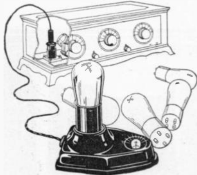
Tube may be tested quickly by attaching the tester to the tube socket of set.
