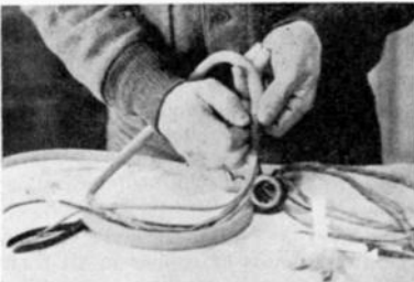
Enclosing all the battery wires in a rubber tube to keep them from a tangle.
