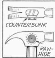
Soft driving head to drive chisels.
