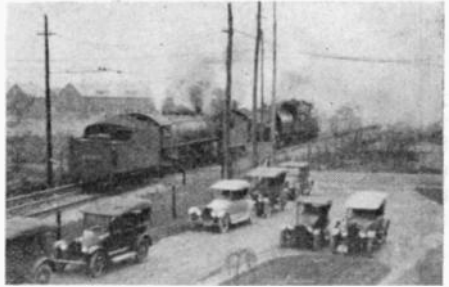
Two steam locomotives placed against an electric engine of the same rated horsepower failed to hold it. The steady pull of the electric power gained advantage over the reciprocating action of the steam engine.
