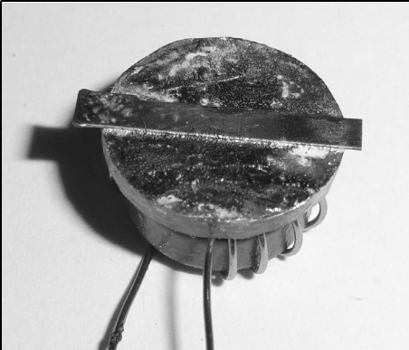
Fig 22: The finished coil is converted into an "SMD component".
