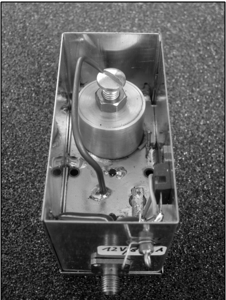
Fig 10: Functional 5GHz cavity oscillator. The thin solid coax phasing line can be seen running along the "cold" side of the PCB.
