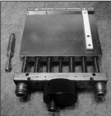
Fig 4: Two so-called "air lines" for adjustment of the phase angle; the path length can be adjusted to 16mm for the SMA version or 24cm for the N type version.
