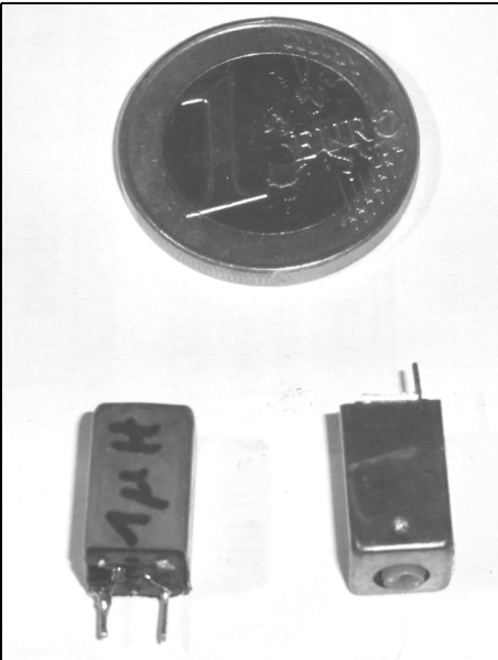
Fig 8: Widely used and proven: the shielded coils from Neosid with a matching core and a size of 7.5 x 7.5mm. Unfortunately a Q no greater than 100 was achieved.
