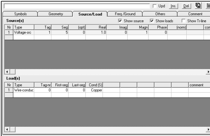
Fig 4: Source/Load tab for definition of source(s), load(s) and lines. Check appropriate combo box to go to sub tab.
