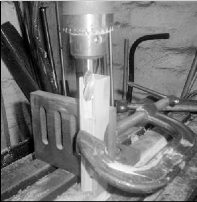
Fig 3: Machining the semicircular element cutouts.
