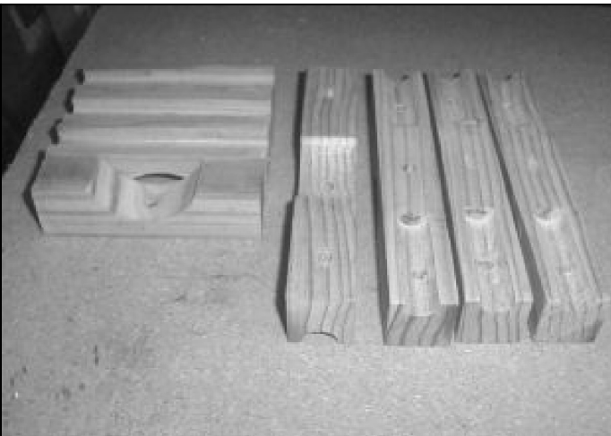
Fig 6: Completed element insulators ready for varnishing.
