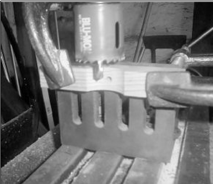
Fig 4: Machining the boom cutout in the bottom of the insulator. The edges of the angle plate allow simple alignment so everything is square.
