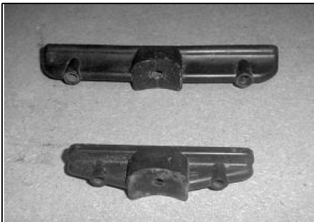
Fig 1: Element insulators for the KLM Yagi. The driven elements use the larger insulators
