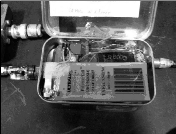
Fig 6: The logarithmic detector AD8307 in its box with battery and output amplifier as described in VHF Communications 1/2004.
