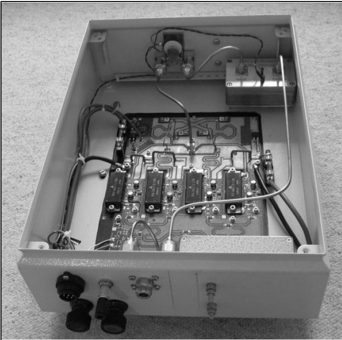
Fig 9: The amplifier mounted in its metal enclosure with a sequencer and a preamplifier.
