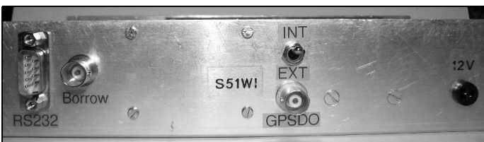
Fig 8: Connectors of the additional unit.
