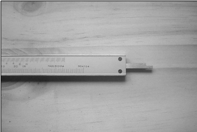
Fig 4: Depth measuring end of a vernier caliper.
