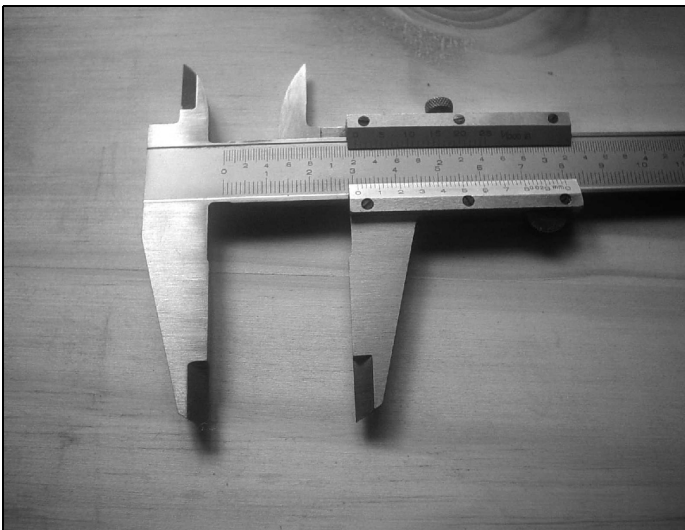
Fig 3: Typical vernier caliper with dual scales.
