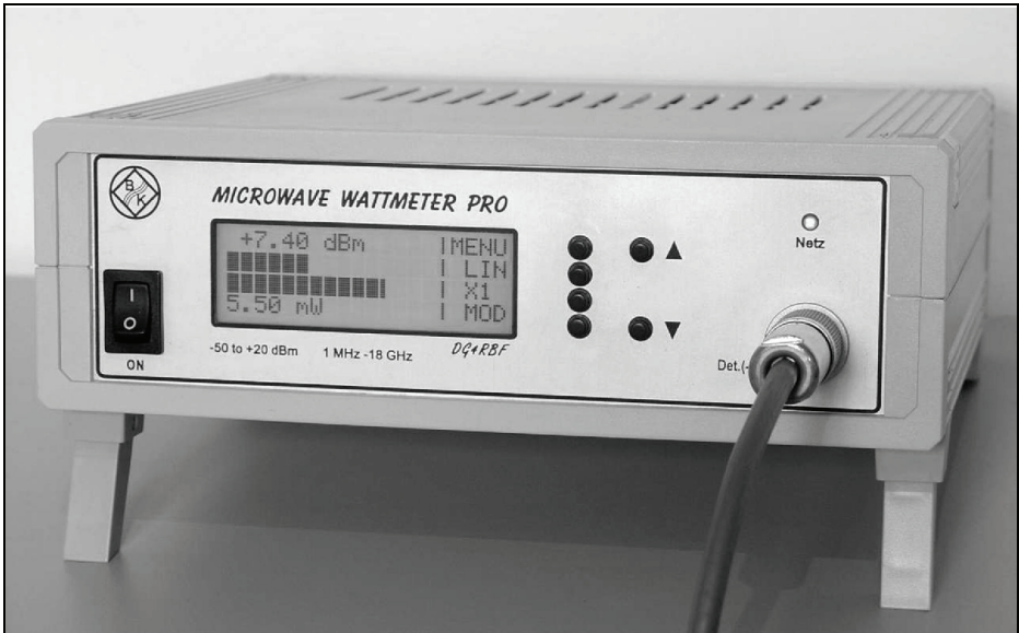
Fig 1: Picture of the completed microwave milliwattmeter.
