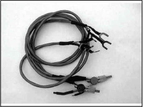
Fig 7: A Kelvin connected pair of test leads from a prime manufacturer, ESI.
