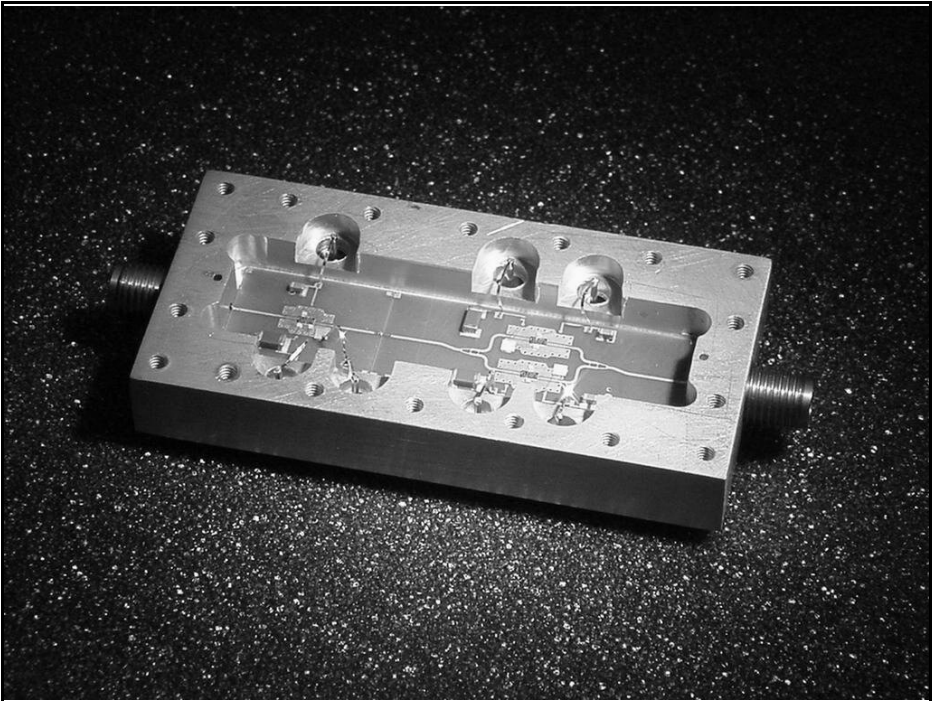
Fig. 2: Assembly of two stage microwave amplifier in gold plated milled housing; the Wilkinson dividers can be easily recognised.
