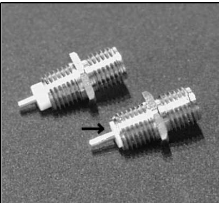
Fig. 11: SMA jacks with unshortened (top) and shortened Teflon edge (below).
