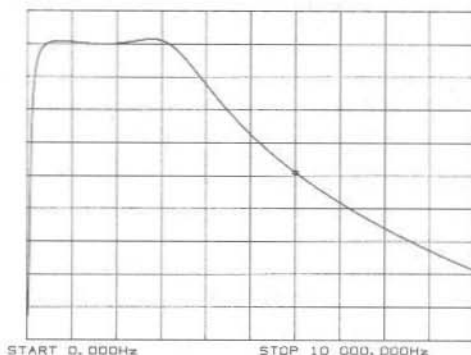
Fig. 9: Measured small-signal frequency response of the speech processor pre-amplifier, dynamic range limiter and band-pass filter.
