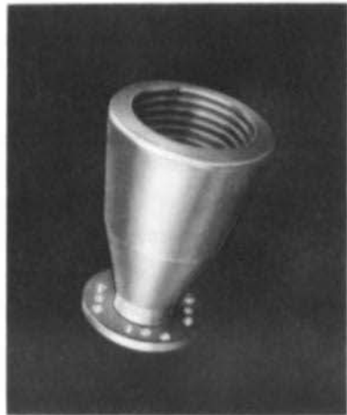
Fig. 9: Laboratory model of a corrugated horn
